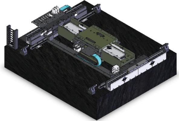
The AHL9000 is the latest addition to Aerotech's family of air-bearing stages and is an excellent choice for applications that require careful balancing of price and performance. This stage has been designed for demanding applications that require excellent step and scan performance. Applications include wafer inspection, flat panel display manufacturing, and optical inspection and fabrication.
