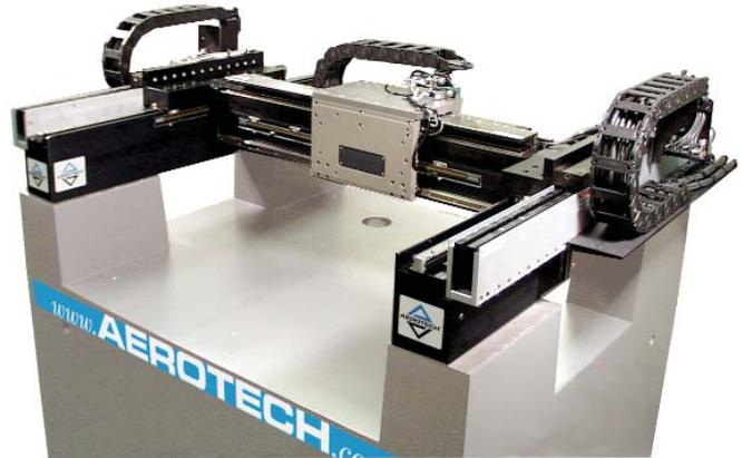
The AGS20000 series was designed to be the most powerful and accurate Cartesian gantry in the world. Dual high-power linear motors were coupled with dual lower-axis linear encoders, resulting in a stage that not only offers unparalleled speeds/accelerations, but is also capable of extreme accuracies and repeatabilities.
